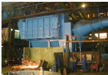
Steel Production Dust removal after flame cutting
