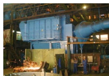
Steel Production Dust removal after flame cutting
